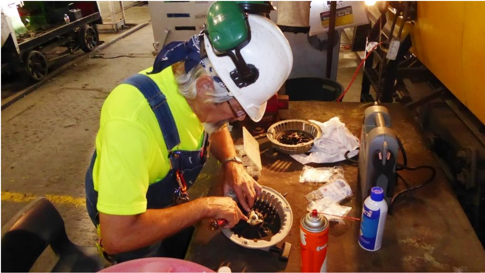
Ed improvises a fix for the gauger's pull-start mechanism
