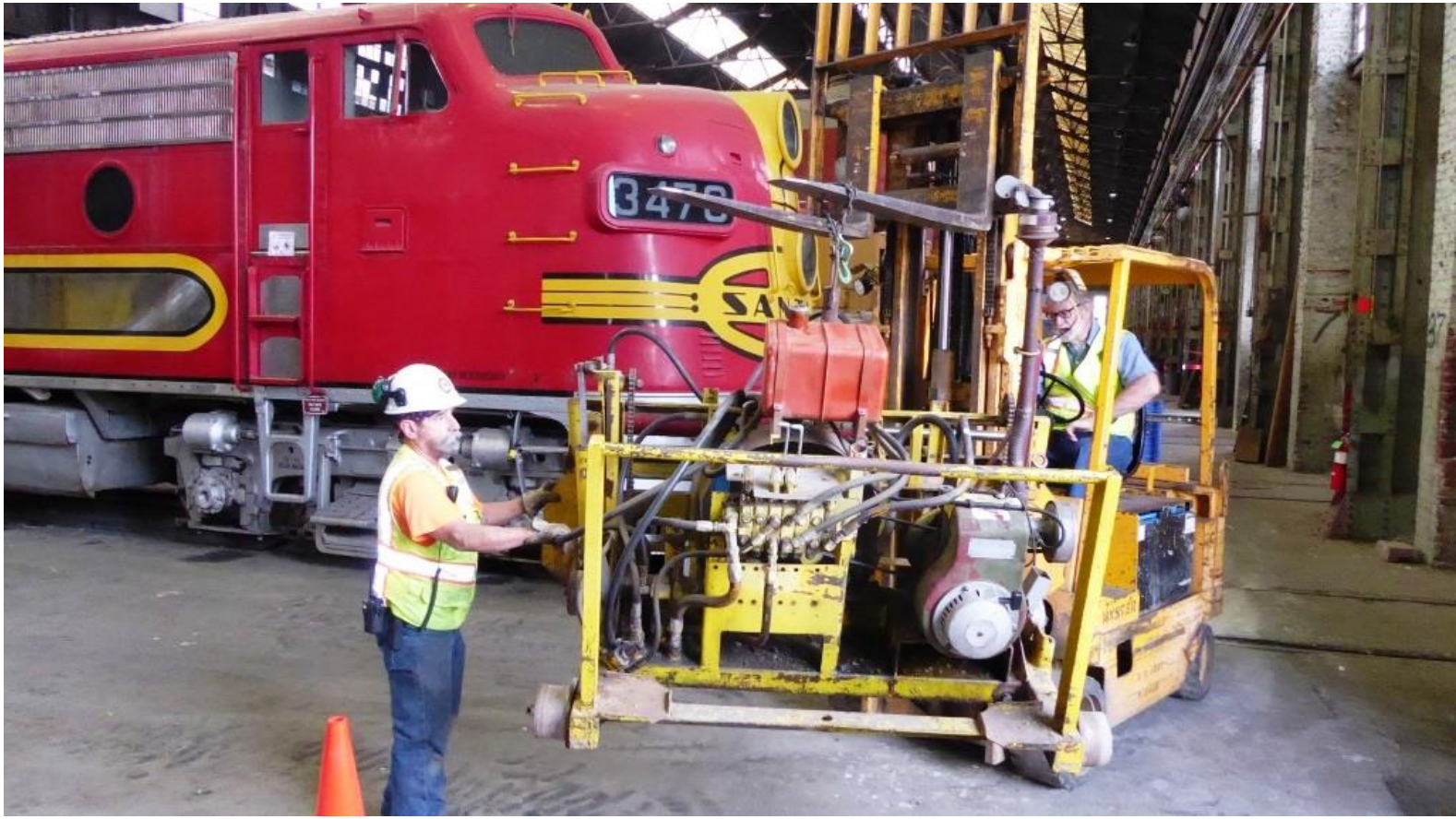
Joe and Alan move the gauger off of its rail-mounted carriage so that it can be used to carry the rail-lifter to the Sutterville Line
